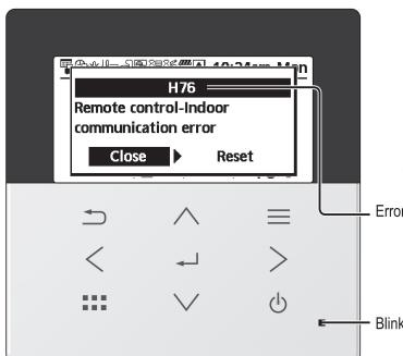
Below is a list of error codes that may appear on the display when there is some trouble with the system setting or operation.
